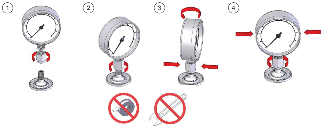
Figure 2. Connecting the Gauge
